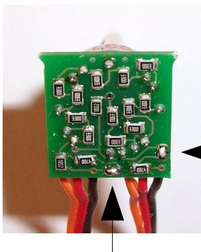
The total resistance of the encoder can be adjusted to your TX by two solder bridges at the rear side of the encoder pcb:
