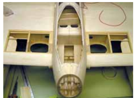
Hornet speaker positions where the radiators would have been
