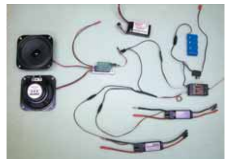
'One Pound Sound' circuit as used in the Beaufighter
