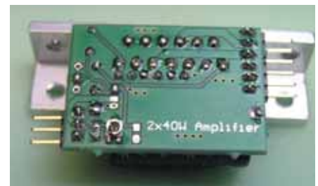
2 x 40 watt amplifier with the volume control on the lower left hand side
