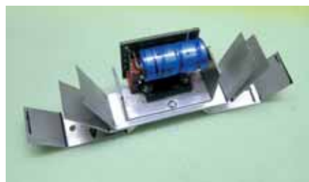
▲ 2 x 40 W amplifier with modified cooling fins
