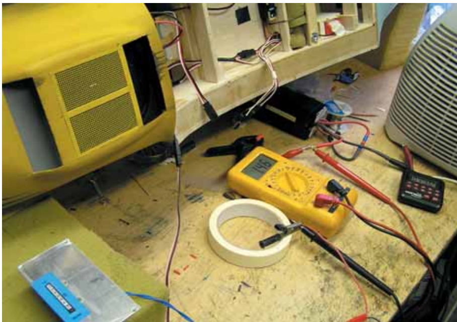
▲ Bench test and running the amplifier is running comfortably cool (with fan on) at 1.5 A
