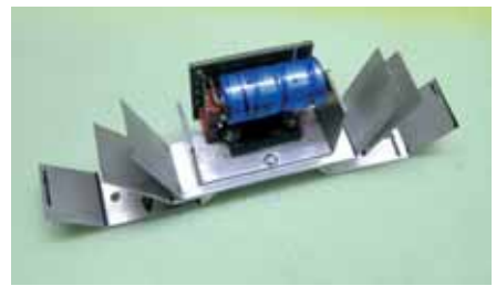
▲ 2 x 40 W amplifier with modified cooling fins
