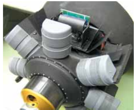
▲ 2 x 40 W amplifier behind the dummy cylinder heads
