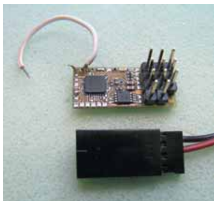
▲ The new TSB4 Micro circuit. All that information held in a circuit the size of a servo connector socket
