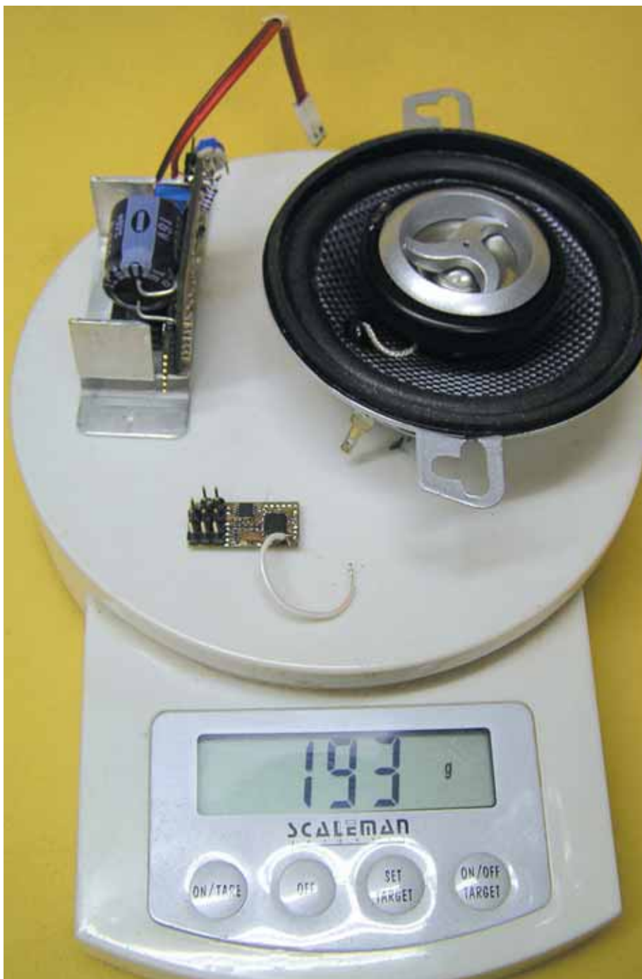
▲ 89 mm Blaupunkt speaker with tweeter. It is hoped to get down to this weight for smaller models
