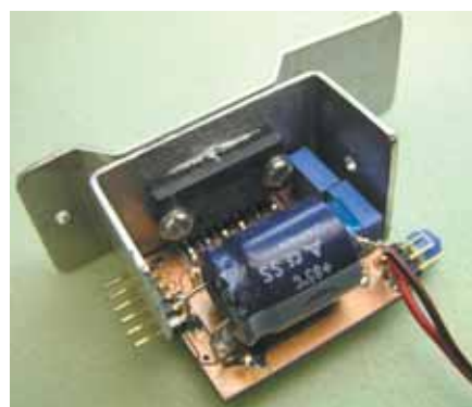
▲ This is a mighty amplifier but it does need the cooling fins to dissipate the heat
