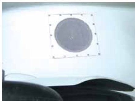
▲ The sound transmits well when it comes from the underside of the wing, the large cavity acts as a sound box
