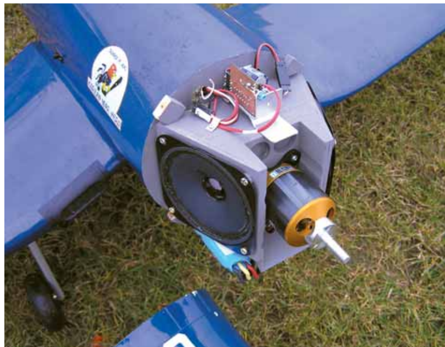
▲ Pete Nicholson's Corsair with the two speakers neatly installed beneath the cowl. The amplifier is well cooled in the air stream
